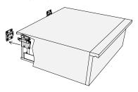
6. Turn the upper screws to adjust the horizontal level.
